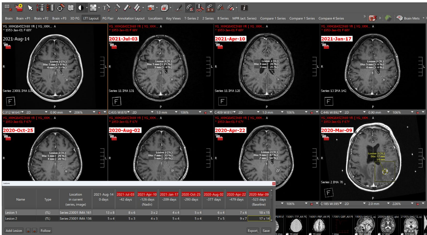
Figure 2. Layout of PACS-integrated AI-enabled BM Lesion Tracking Tool Eight co-registered series of T1 gadolinium-enhanced sequences are depicted, while the implemented hanging protocol and LTT layout feature are activated. Within the shown lesion tool card, two identified metastases and their AI-generated maximum orthogonal diameters, highlighted on each series, are matched and longitudinally aligned. Visualized on the corresponding images, the AI-LTT provides automated critical information regarding the individual behavior in size and treatment response of each lesion over up to eight study dates.
